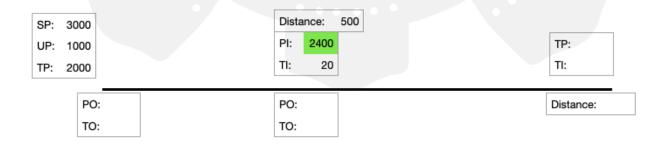
With an interval of 150 we can anticipate that we will hit our TP of 2000psi at about minute 33 UP/interval X 5 = TI 1000/150 X5 = TI 6.6 X 5 = 33.33
